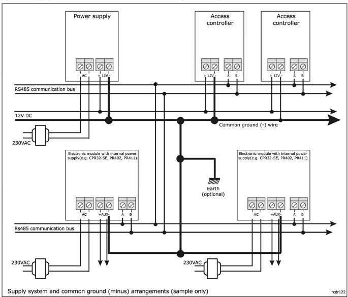
Note: It is forbidden to short positive (+) supply outputs from various devices working in the system.
