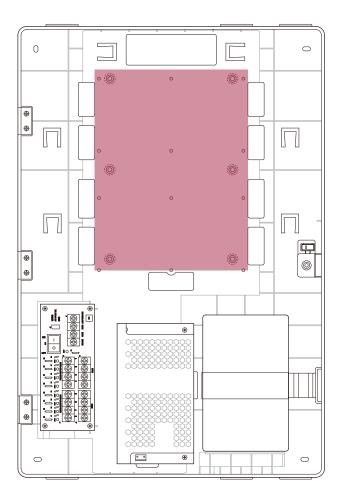
**2** After positioning CoreStation in the enclosure, fix it with the fixing screws.
