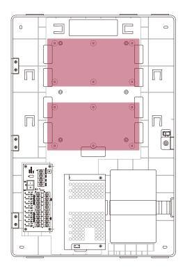
**2** After positioning the Output Module in the enclosure, fix it with the fixing screws.
