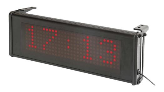
The ASCD-1 is a five segment LED matrix display. In RACS 4 the device can display system time in 24h format while in RACS 5 it can additionally display system text messages with maximal length of 32 characters. When the text is longer than matrix (5 characters) then it is smoothly scrolled. Alternatively the ASCD-1 can be used beyond RACS systems as a standalone clock using internal RTC or as a display presenting received text messages. The device can additionally display ambient tempe-
