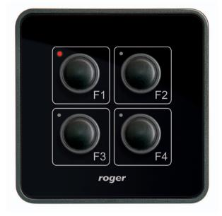
HRT82PB panel provides four momentary type buttons with insulated NO contacts and four externally controlled LED indicators. The NO contact can be used to trigger controller's input while LEDs to indicate state of controller's outputs. Panel can be used in other scenarios as long as its nominal electrical condition is assured.
