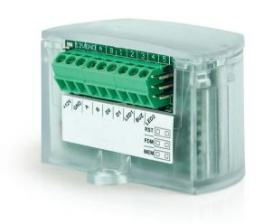
The interface enables the connection of the MCT series reader (RACS 5 system) to controllers that use the Wiegand protocol. The interface works as a communication converter from the RS485 EPSO 3 protocol to the Wiegand data transmission standard.
