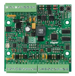
The MCX2D is an 2 door IO expander dedicated for the RACS 5 system. Apart from the IO lines, it distributes power supply and RS485 communication bus to the controlled doors. For each door it provides 2 signal inputs, 2 control outputs, 2 supply outputs and communication interface to readers. The door circuits are electrically separated what assures that in case of malfunction or sabotage, the problem which occurred on single door is not propagated to other doors. The MCX2D is supplied
