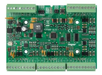
The MCX4D is an 4 door IO expander dedicated for the RACS 5 system. Apart from the IO lines, it distributes power supply and RS485 communication bus to the controlled doors. For each door it provides 2 signal inputs, 2 control outputs, 2 supply outputs and communication interface to readers. The door circuits are electrically separated what assures that in case of malfunction or sabotage, the problem which occurred on a single door is not propagated to other doors. The MCX4D is supplied
