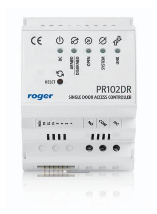
PR102DR access controllers may operate as standalone access control units or in integrated access control system with CPR network controllers. In standalone mode PR102DR autonomously supervise two-way door passage and do not need to communicate with PC nor any other equipment, events are registered in their inter-
