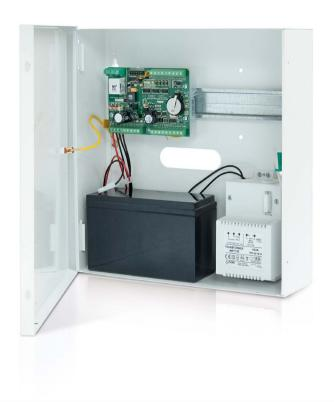
PR411DR-SET consist of PR411DR-BRD access controller module and TRP 40/16/18 power transformer factory preinstalled in ME-1 metal enclosure with space for 7 Ah/12 V back-up battery and tamper contact.
