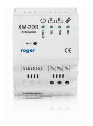
XM-2DR is an I/O expander dedicated to systems using RACS CLK/DTA protocol. Expander offers two NO/NC inputs and two relay outputs with 1.5 A/30 VDC and 5 A/30 VDC max load respectively. Optionally, XM-2DR can be used as a standalone device (without communication with master device), when so, its outputs are controlled by signals applied to its inputs.
