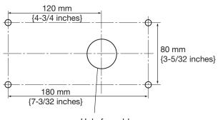
Hole for cable installation: ø38 mm {ø1-1/2 inches}
