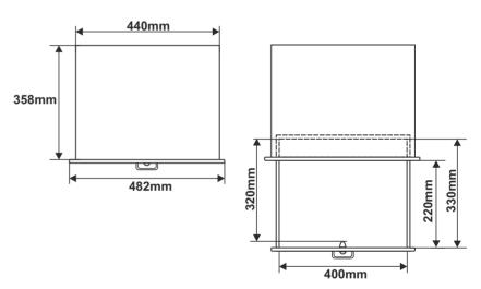
**INTENDED USE**The 2U high RACK drawer is intended for storing / mounting supplementary elements in RACK cabinets.
