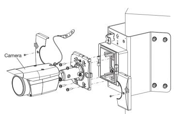
d) Use one M6 hexagon screw (accessory) to fix the safety wire of the camera onto the safety wire fixing bracket (accessory).
