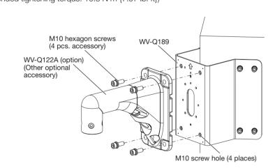
• When install WV-Q185 (Wall mount bracket: Light gray), please use WV-Q183 (Light gray). When install WV-Q122A (Wall mount bracket: Fine silver), please use WV-Q189 (Fine silver). **B** Install network camera with round camera mount bracket <WV-Q189>
