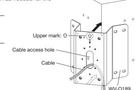
4 Use eight M8 screws (locally procured) to install WV-Q189 onto the corner. Minimum pull-out strength: 823 N {185 lbf} (per 1 pc.)
