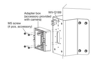
c) Mount the camera onto adapter box (accessory provided with camera) please refer to the manual
