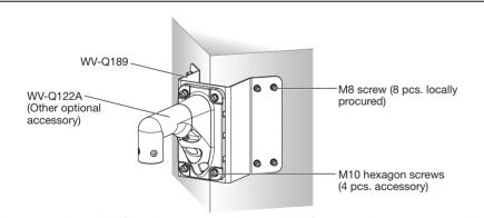
(In this illustration, fixing WV-Q122A to a corner by using WV-Q189 is taken as an example.
