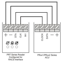
When employing RACS transmission format, the PRT62 unit communicates with its host ACU via the CLK and DTA lines. Unlike in the Wiegand or Magstripe formats, the PRT62 unit using RACS format requires an individual address (ID=0...3) to be set for it during configuration of the reader.
