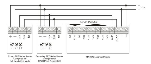
The max. cable length between a PRT reader and an XM-2 module or between a primary and a secondary PRT reader units is limited to 150 m. For two-way door control, the primary PRT unit needs to be configured for **Full Stand-alone Mode** and the interconnected secondary PRT unit needs to be configured for **RACS Mode** with its device address set to ID=0.
