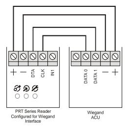
When employing Wiegand transmission format, the data are transferred using sequences of pulses sent over the CLK and DTA lines. Depending on the selected version of the transmission format, the PRT reader uses 26, 34, 42 or 66 bits to transmit a code read in from the card presented or the PIN code entered.
